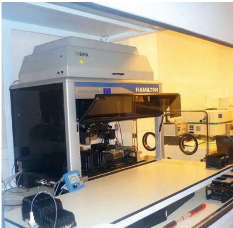
▲ The parts of the Cocagne automated platform for culture and isolation of microbes (IUEM): fluid-handling robot, anaerobic chamber and flow cytometer
